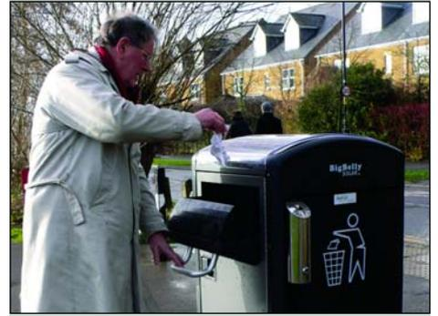
Meet Oxford city's brand new **solar powered waste bin**. Each one is wired up to measure waste levels inside. When there's enough to compress, it is solar powered to do that, and then, when it is nearly full an alert is sent electronically to [recycling@Oxford](mailto:recycling@Oxford) to say it's time to collect. A really smart bin!
